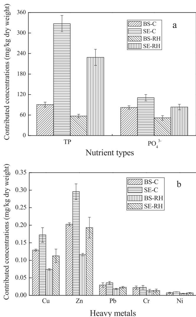
Fig. 6. The contributed concentrations of (a) potential nutrients retention about TP,  $PO_4^{3-}$  and (b) heavy metals immobilized for final composts.
