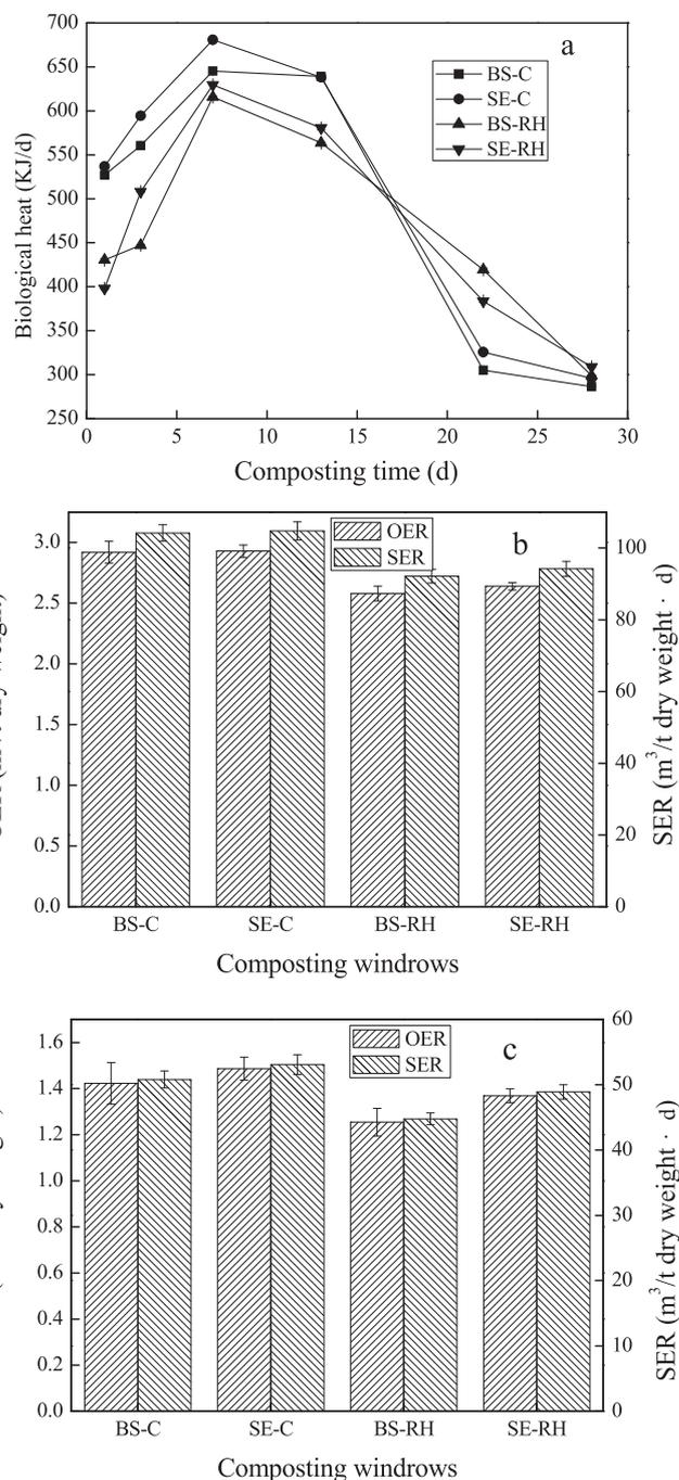
Fig. 4. The characteristics of (a) biological heat generation, (b) OER and SER for water balance during the whole composting process and (c) OER and SER for LM-only consumption during the composting process.
