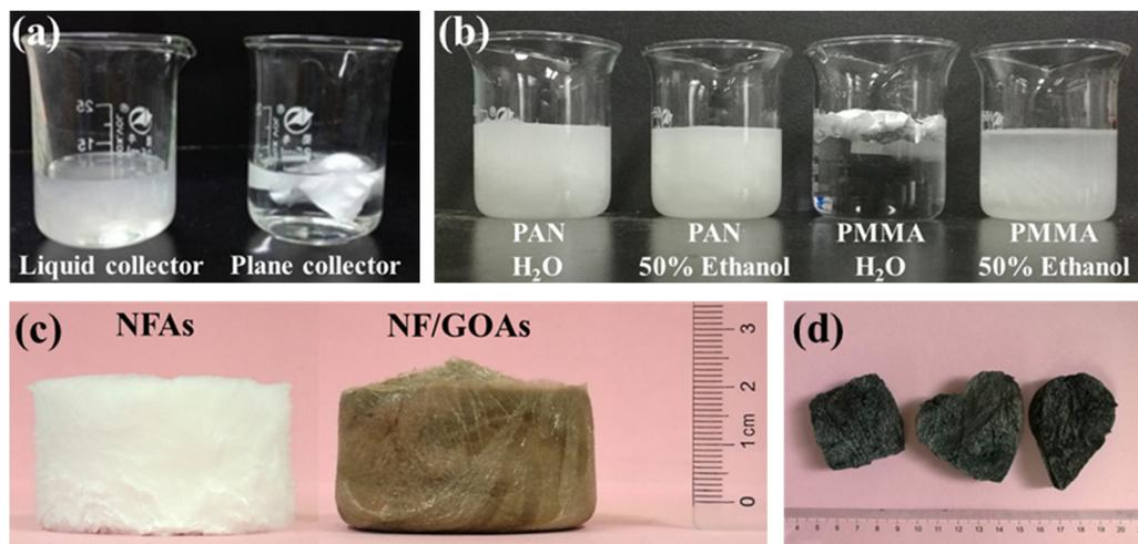
**Fig. 2.** Analysis of 3D aerogel architecture building requirements and optical photographs of the aerogels in preparation process. (a) Different dispersibility of PAN nanofibers collected by deionized water and 2D PAN nanofibrous membrane in deionized water. (b) PAN and PMMA nanofibers showed different dispersibility in pure water and 50% ethanol. (c) An optical photograph of NFAs and NF/GOAs. (d) An optical photograph of resultant CNF/GOAs in diverse shapes.
