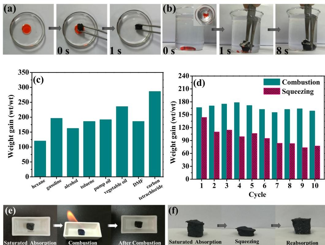
**Fig. 6.** Oils absorption properties of the hydrophobic CNF/GOAs. The absorption processes of the hydrophobic CNF/GOAs toward (a) toluene on water surface and (b) carbon tetrachloride underwater. (c) Absorption capacity of CNF/GOAs toward diverse oils. (d) Cyclic absorption capacity of CNF/GOAs toward ethanol, which recycled with combustion and squeezing methods, respectively. Regenerate process of CNF/GOAs after saturated absorbing ethanol by (e) combustion and (f) mechanical squeezing.
