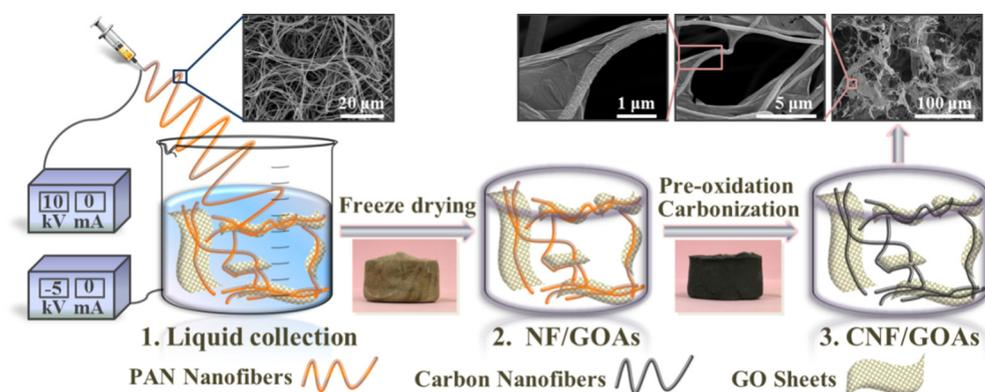
**Fig. 1.** Schematic diagram shows the main preparation procedure of CNF/GOs: (1) continuous electrospun PAN nanofibers were collected by GO aqueous dispersion; (2) 3D NF/GOAs were prepared by freeze drying the PAN nanofibers/GO sheets aqueous dispersions; (3) CNF/GOAs were prepared by thermal treatment of NF/GOAs including pre-oxidation and carbonization.
